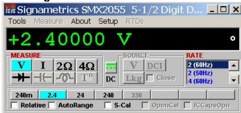
Figure 3-2. The Control Panel. The three main groups include Measure, Source and Range buttons. The Range buttons are context sensitive such that only “240m, 2.4, 24 and 240 appear when in AC Voltage Function is selected, and 2.4m, 24m, 240m and 2.4 appear when AC Current functions is selected, etc.
